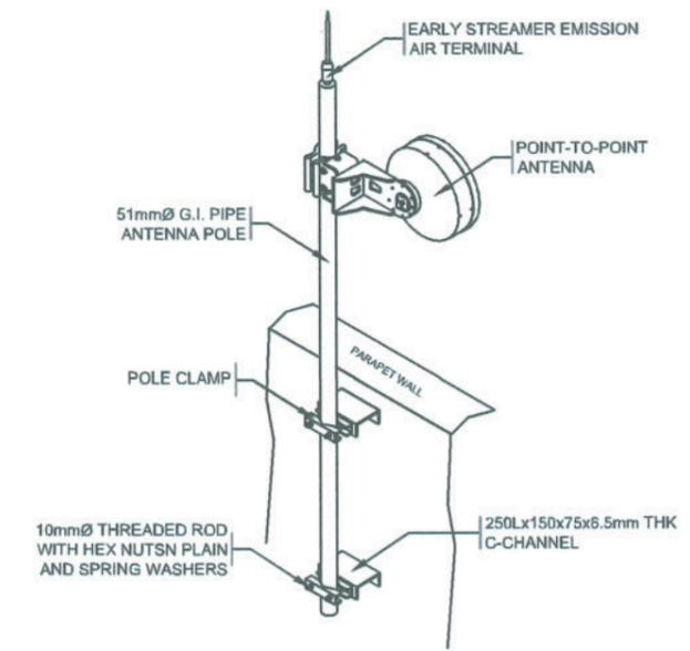
**DETAILS OF POLE FOR EARLY STREAMER EMISSION AIR TERMINAL AND ANTENNA**
